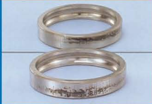
Phenomenon: Symmetrical Fretting on Upper and Lower Sides
