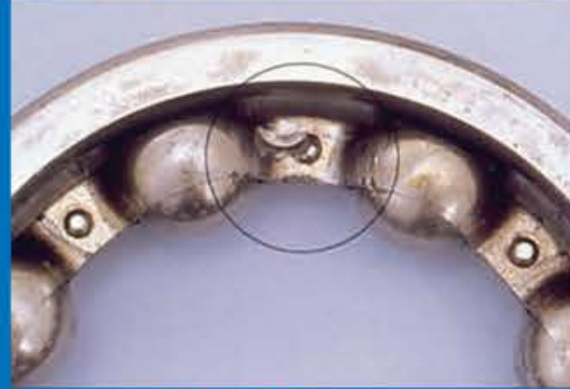
Phenomenon: Dents on Retainer
