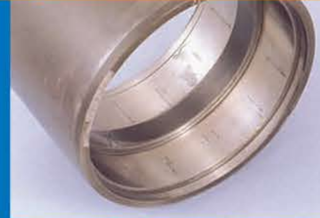
Phenomenon: Rust Generated on Raceway at Intervals on Roller Pitch
