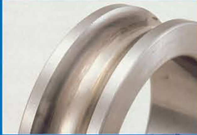
Phenomenon: Smearing on Raceway
