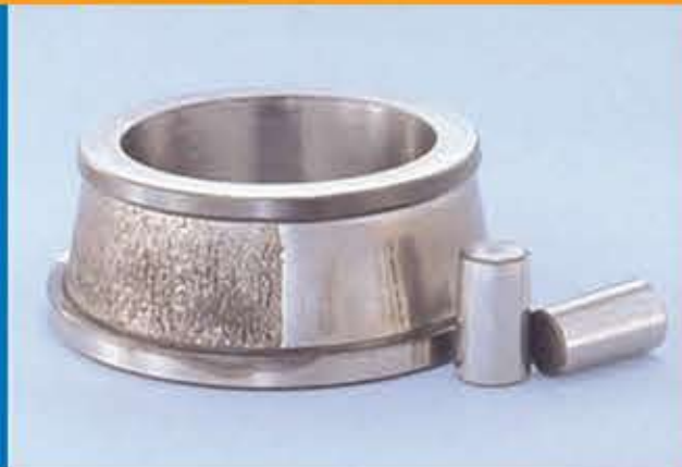
Phenomenon: Flaking Generated Around Half the Raceway
