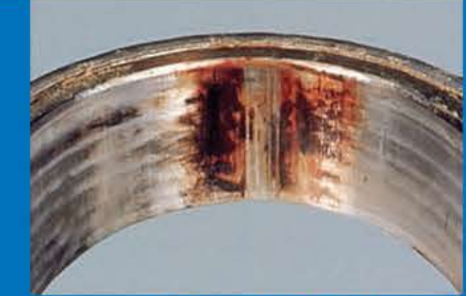
Phenomenon: Scuffing on Bore Surface
