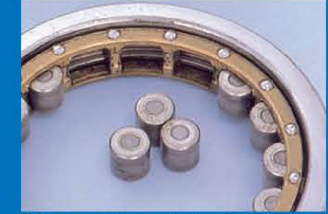
Phenomenon: Wear on Retainer Pocket Surface/Guide Surface
