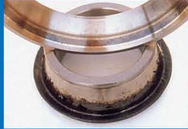
Phenomenon: Seizure at Roller End Surface and Inner Ring Rib
