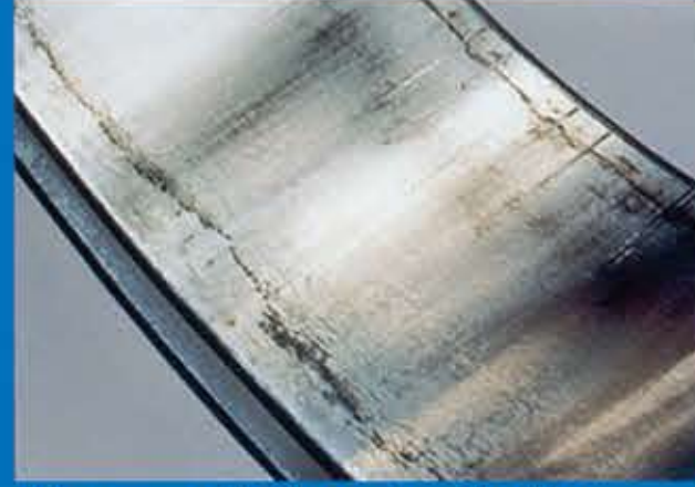
Phenomenon: Scuffing on Inner Ring Bore Surface
