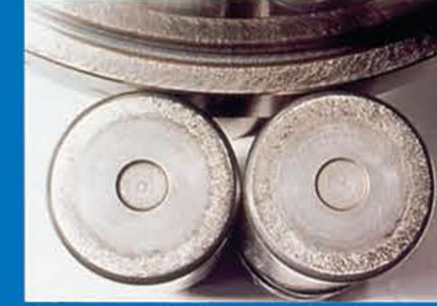
Phenomenon: Scuffing on Roller End Surface and Inner Ring Rib
