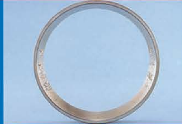
Phenomenon: Flaking on Opposite Faces of Raceway
