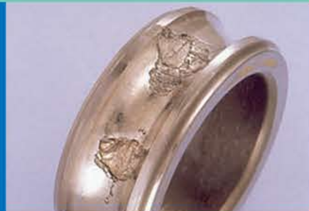
Phenomenon: Flaking at Intervals on Ball Pitch
