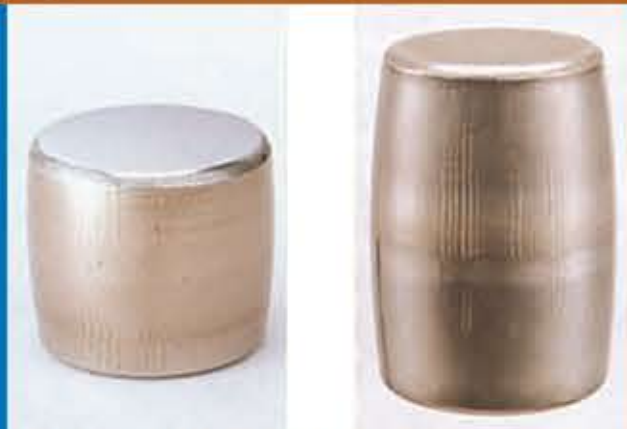
Phenomenon: Electric Pitting (Pit or Ridge) and Staining
