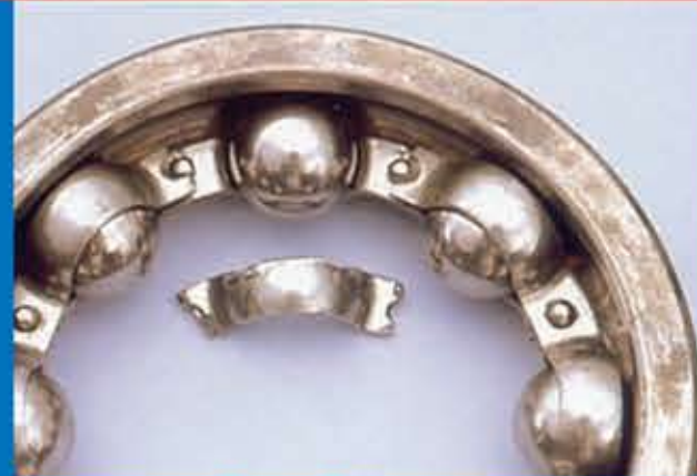
Phenomenon: Broken Retainer
