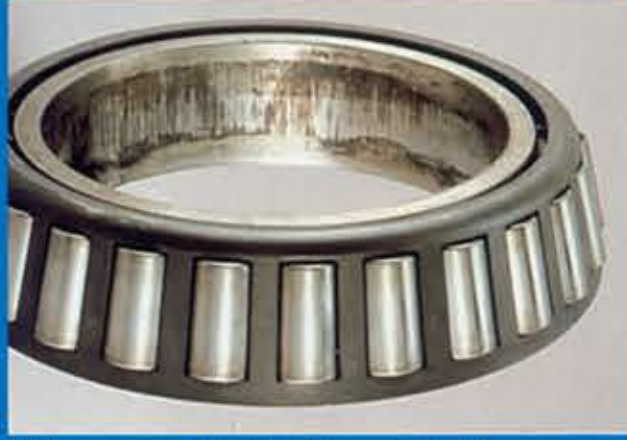
Phenomenon: Fretting Corrosion (Left)
