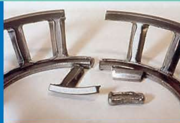
Phenomenon: Broken Retainer
