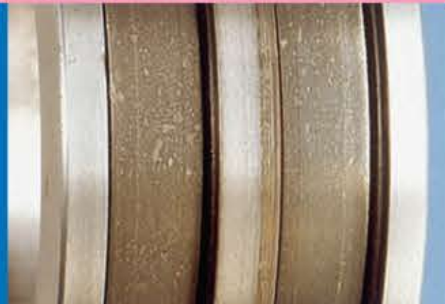
Phenomenon: Indentations on Raceway
