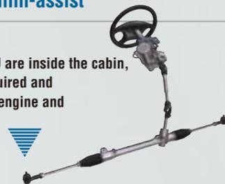
Optimum steering system for compact vehicles with small rack force
